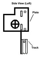
Track position can vary, but should never be closer than 3/4" from the glass or any other obstacle. Before installing track, wipe mounting surface with dry cloth, use isopropyl alcohol if needed. Install track using pre-applied double-face tape.
